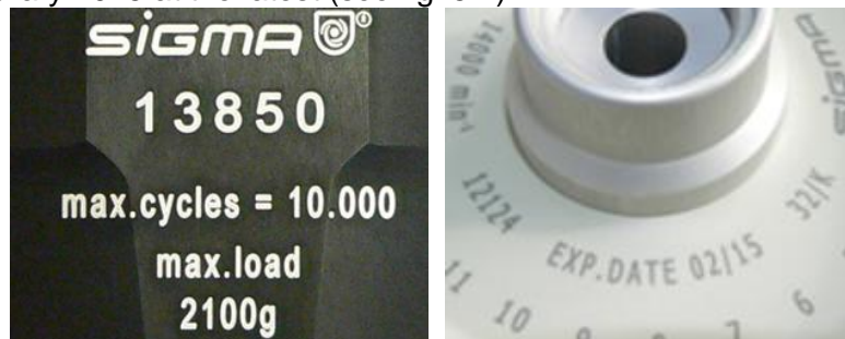
Fig. 5.7: Different service life – engraving on the bucket/rotor
