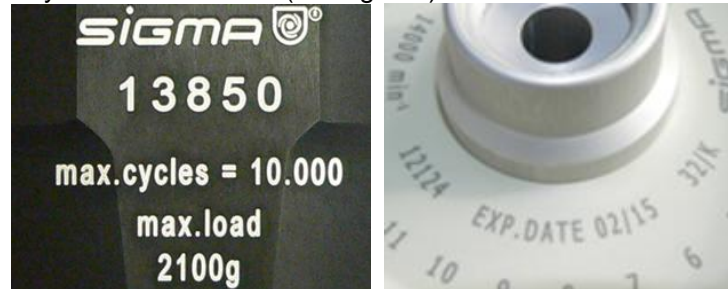
Fig. 5.9: Different service life – engraving on the bucket/rotor
