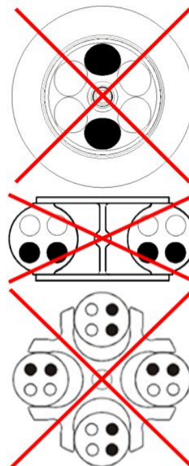
Fig. 7: Permissible and impermissible loading of an angle rotor and a swing-out rotor (example illustrations)
