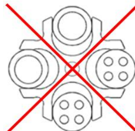
Fig. 6: Permissible and impermissible loading of a swing-out rotor with different tube sizes (example illustration)
